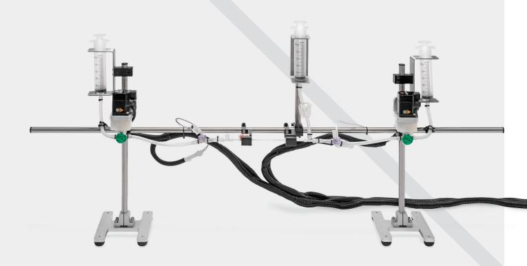
Our MicroMaxx tangential flow filtration (TFF) systems are designed specifically for benchtop TFF applications and hollow fiber filter screening.
