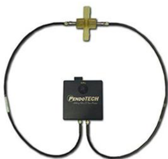
Photo 1: Assembled UV flow cell, optical couplers, fiber optic cables, and photometer/transmitter
