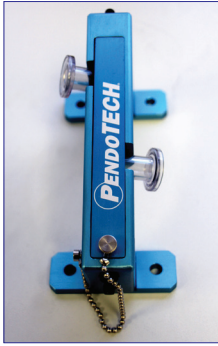
6.5cm flow cell installed in stand
