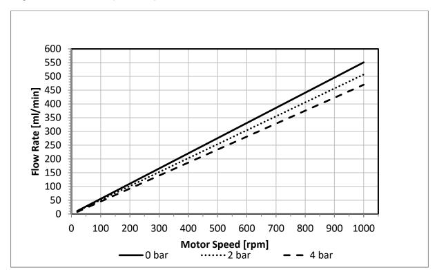
The flow rates showing at the chart above were ascertained with a new pump chamber under standard conditions after the final assembly of the pump.
