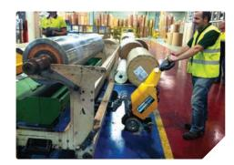
Our SmartMover range is suited to all industries, including the most challenging environments or confined spaces. Using a leveraged weight transfer system and dual drive motors, this compact tug generates enough power to move loads weighing up to 2,600 lb. The coupling points are cleverly designed to attach to loads quickly whilst providing a safer, unbreakable connection. A two speed switch and an anti-crush button are also provided as standard.
