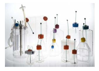
CITSens *Bio* sensors are based on screen printed electrodes which are coated with an immobilized enzyme. The sensor is built into the respective original cap or finished as a PEEK PG13.5 sensor, double packaged and subsequently sterilized by gamma-irradiation.
