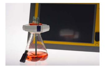
CITSens *MeMo* is an electrochemical, enzymebased sensor system with the capacity to be used in defined cell culture media as well as in complex matrices, e.g. blood.
